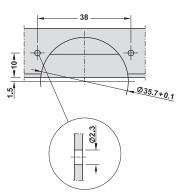
Metalla 510 Cruciform Mounting Plate -With Quick Fixing System
