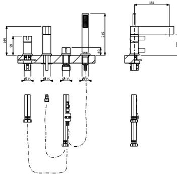
**589.80.134**- Four-hole deck mounted bath mixer with diverter and pull-out handshower
