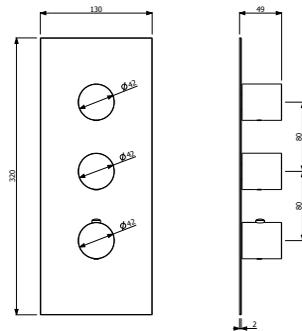
**589.80.921**- External part of thermostatic concealed high-flow rate mixer with 2-way diverter
