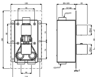
**589.80.923**- External part of thermostatic concealed high-flow rate mixer with 1-way diverter
