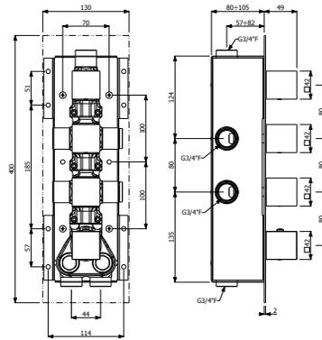
**589.80.925** - External part of thermostatic concealed high-flow rate mixer with 3-way diverter
