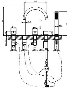
**589.80.219**- Five-hole deck mounted bath mixer with diverter and pull-out handshower
