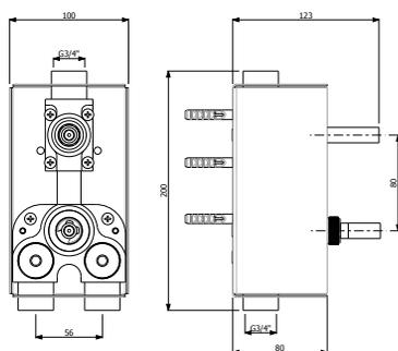
**589.80.910**- Concealed part of thermostatic concealed high-flow rate mixer with 1-way diverter
