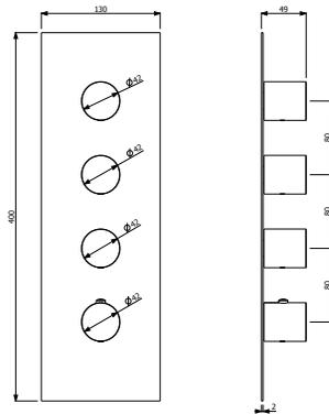
**589.80.922**- External part of thermostatic concealed high-flow rate mixer with 3-way diverter
