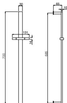
Sliding Rail (25mm width x 750 mm length) with minimal design brackets and front loading slider mechanism 75 cm
