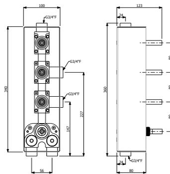
**589.80.912** - Concealed part of thermostatic concealed high-flow rate mixer with 3-way diverter
