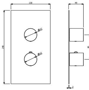
**589.80.920**- External part of thermostatic concealed high-flow rate mixer with 1-way diverter
