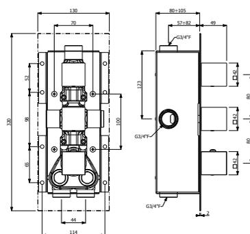
**589.80.924**- External part of thermostatic concealed high-flow rate mixer with 2-way diverter
