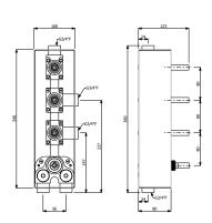
**589.80.912** - Concealed part of thermostatic concealed high-flow rate mixer with 3-way diverter
