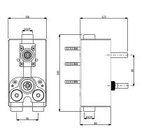
**589.80.910**- Concealed part of thermostatic concealed high-flow rate mixer with 1-way diverter
