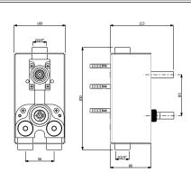
**589.80.910**- Concealed part of thermostatic concealed high-flow rate mixer with 1-way diverter
