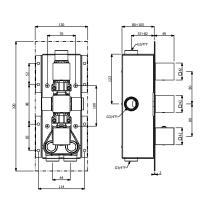
**589.80.924-** External part of thermostatic concealed high-flow rate mixer with 2-way diverter
