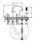
**589.80.219-** Five-hole deck mounted bath mixer with diverter and pull-out handshower
