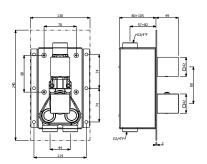
**589.80.923-** External part of thermostatic concealed high-flow rate mixer with 1-way diverter
