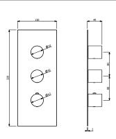
**589.80.921-** External part of thermostatic concealed high-flow rate mixer with 2-way diverter
