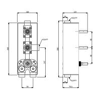
**589.80.911**- Concealed part of thermostatic concealed high-flow rate mixer with 2-way diverter
