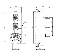
**589.80.911-** Concealed part of thermostatic concealed high-flow rate mixer with 2-way diverter
