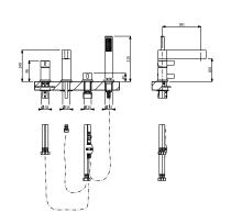
**589.80.134-** Four-hole deck mounted bath mixer with diverter and pull-out handshower
