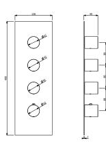
**589.80.922-** External part of thermostatic concealed high-flow rate mixer with 3-way diverter
